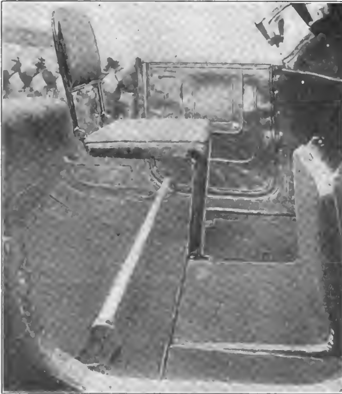
Illustrating the manner in which the auxiliary seats in the tonneau of the seven-passenger Overland six fold into the back of the front seat
